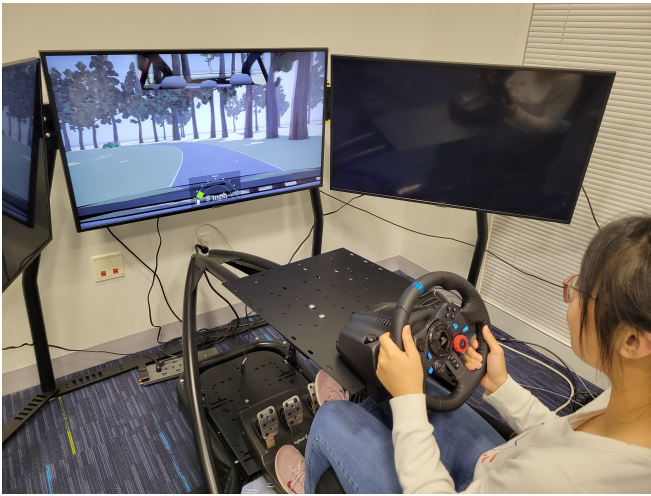
Fig. 4: A participant using the driving simulator to control the ego vehicle
